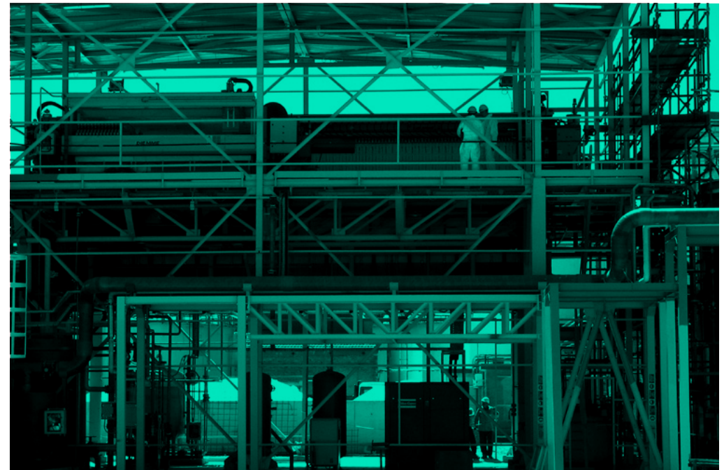
Figure 7: Diemme® Filtration ME1000 used for the separation of Mg hydroxide from \text{CaCl}_2
