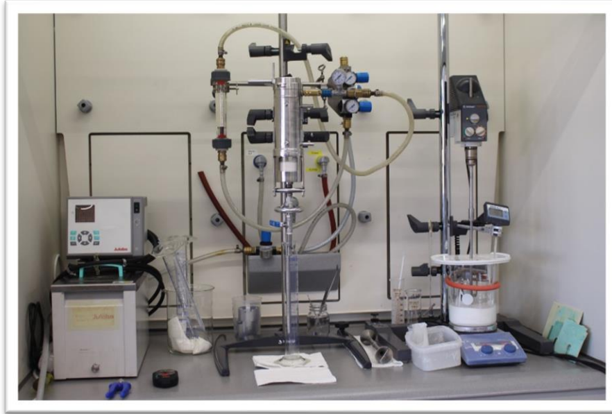
FIGURE 1: PRESSURE FILTRATION TESTING (COURTESY OF BHS-SONTHOFEN INC.)
