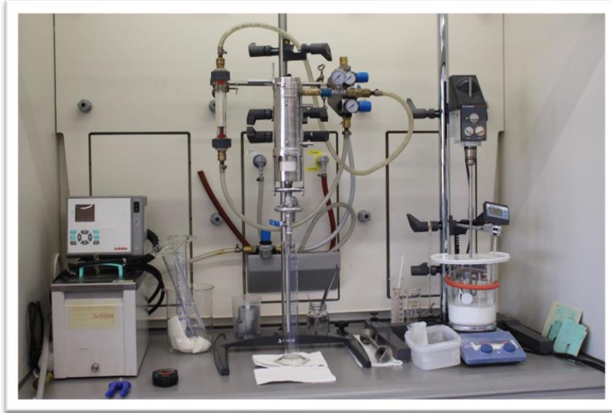
FIGURE 1: PRESSURE FILTRATION TESTING (COURTESY OF BHS-SONTHOFEN INC.)
